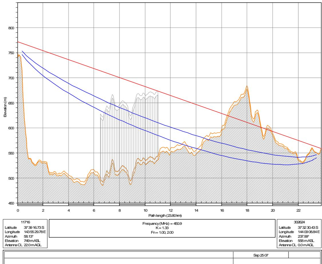
The Fresnel zone of interest is along the path from the Mt Buninyong site to the knife edge obstruction. This section of the path is shown in the following Figure. The first Fresnel zone of this path is smaller, as the path length is shorter.
