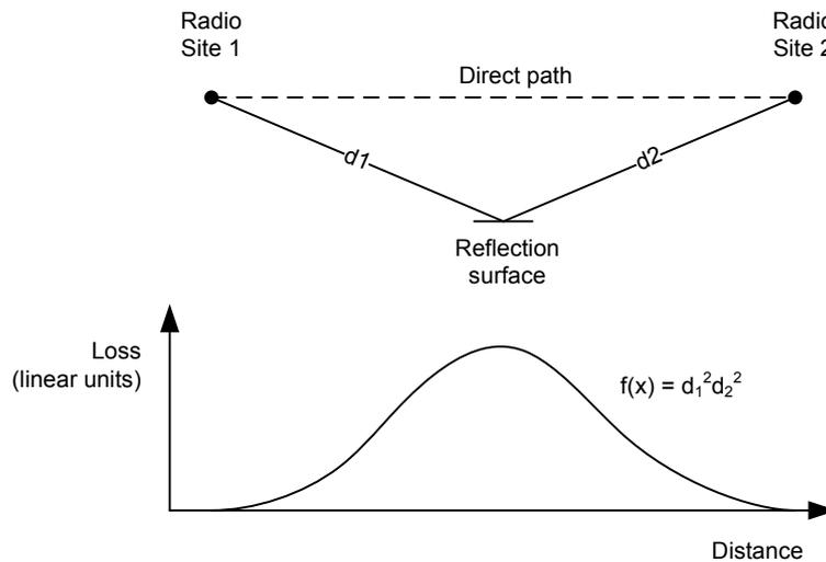
Figure 2.3 – Transmission over an indirect path
