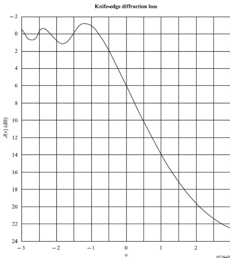
Figure 2.2 – Knife edge diffraction loss from ITU-R P.526-10
